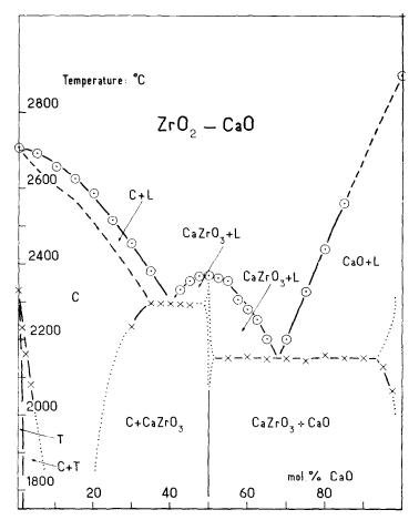
FIG. 6. Phase diagram of the ZrO<sub>2</sub>-CaO system as seen by Traverse and Foex (5).
